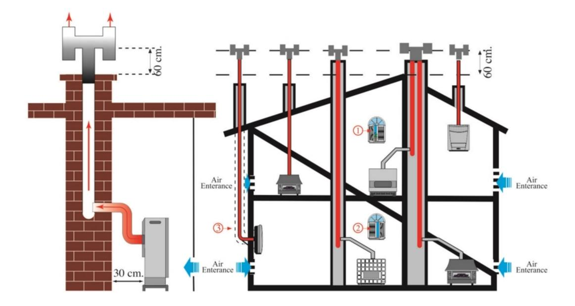
Since the required air for the operation of this type of gas heater is provided from inside the building, so the building or the room that gas heater is installed should have a proper ventilation system in a way that fresh air flow inside easily.
