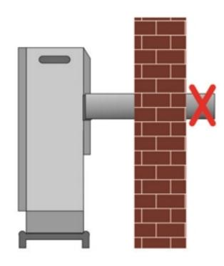
Ounder no condition the level of the chimney inside the building should not be lower than the level of the heater pipe. Otherwise the installation of the heater by the servicemen will be prohibited, unless an authorized person makes it correct.
