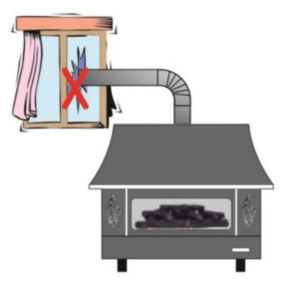
Seach heater should have its independent chimney, so do not connect more than one heater or other gas, oil or gasoline utilizations to one chimney.
