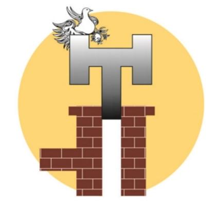
The chimney of the heater inside the building should not be placed horizontally and should have a minimum 45-degree angel from the floor of the room.
