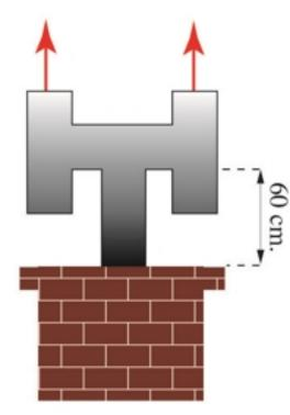
If a gas heater is installed in a building near higher buildings, so the height of the chimney should be 60 centimeters higher than the roof of the highest building.
