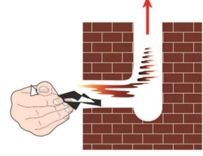
**○** If the chimney of the building is not proper for installation, the servicemen should not install the heater, unless an authorized person corrects the chimney of the building.
