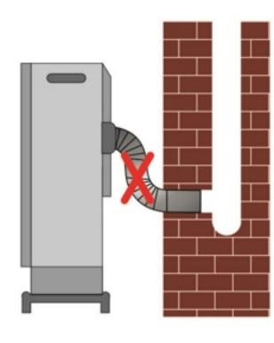
On not pass the chimney pipe from the glass of a window since the chimney become warm so the glass may be cracked or broken and the heater chimney will be fall down.
