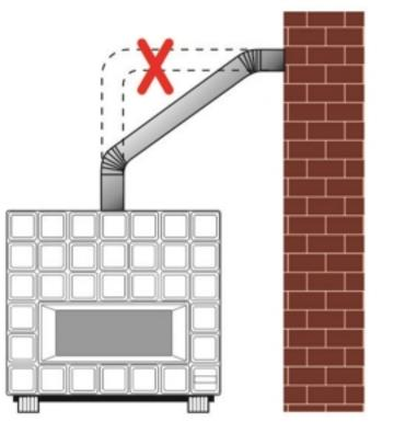
One of the correct operation signs of a heater chimney system and a building chimney is that when heater operates (maximum 5 minutes after operation) the metal chimney will become warm. So it is better to check the heater chimney sometimes to be sure it is warm.
